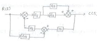
(d) Draw signal flow graph and find C(s)/R(s) by using Mason's gain rule.
